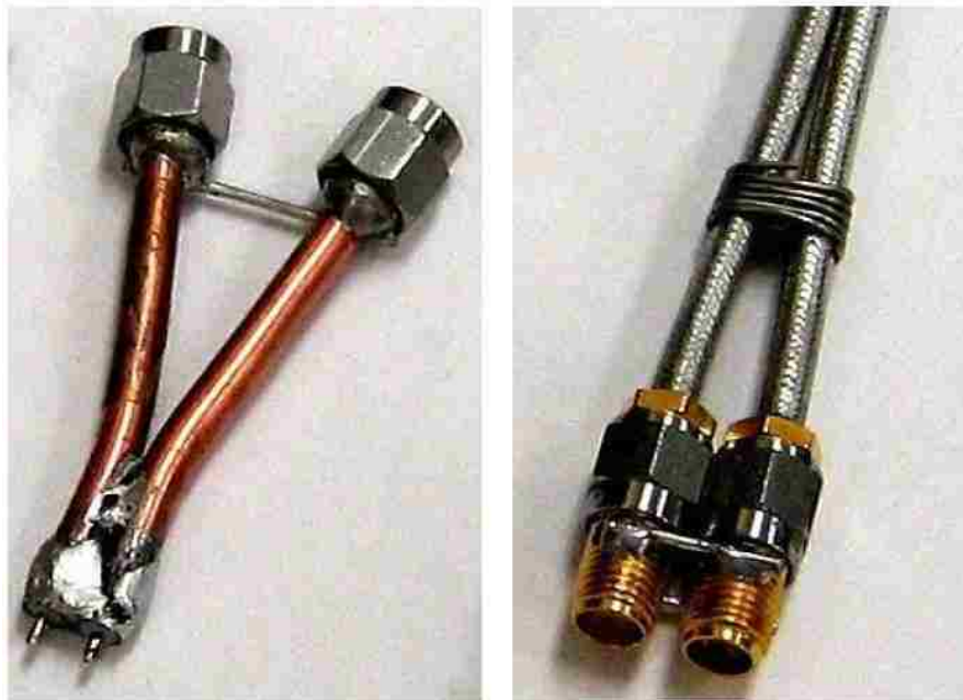
Figure 6-2. Differential measurement jigs, Koskinen et al. use the right jig to measure differential antennas, including unbalanced. Picture from Koskinen et al. [43].
