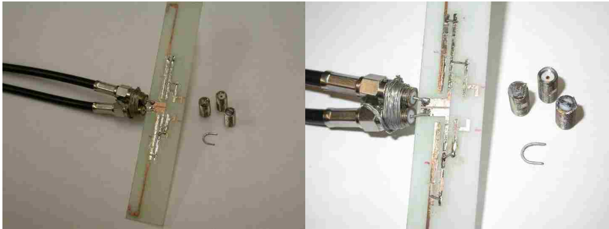
Figure 6-3. Port 1 and Port 2 coax cables combined into a differential probe, with the ability to disassemble for SOLT calibration without having to de-embed a separate probe. Prototype calibration standards are made using 3 barrels and a C-shaped wire as a through standard. This antenna is tuned for 50 Ohm.
