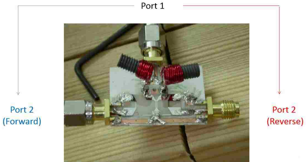
Figure A-6. A low frequency, 40MHz, test structure for verification of equation A-3, and proof of operation before continuing to work at higher frequency.
