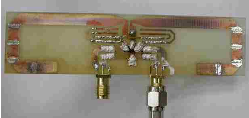
Figure A-14. 1 st attempt at wireless operation using a folded dipole antenna and the phasing topology in Figure A-3. Proper phasing of the inductors was not successful and a new phasing topology was adopted (Figure A-15).
